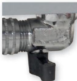
1. Control valve of steam jacket
