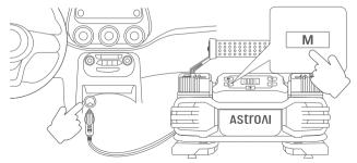
2. Press the "M" Button to choose the desired unit (4 options: PSI, Bar, kPa, kg/cm²).
