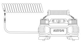
Remove the cap from the tire's valve stem, connect the air hose nozzle to the valve stem. (Tips: For better sealing when using the quick connector, align it to the valve stem, firmly press it in and flip the small lever.)
