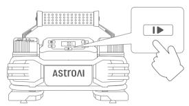
Press and hold the "M" Button for 3 seconds to turn off the air compressor after inflation.
