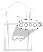
Press the Power button on the back of the speaker to turn it on. The indicator light on the front of the speaker blinks while the speaker is tuning to the transmitter. The indicator light turns solid blue when the speaker is tuned to the transmitter-you should hear sound coming from the speaker now.
